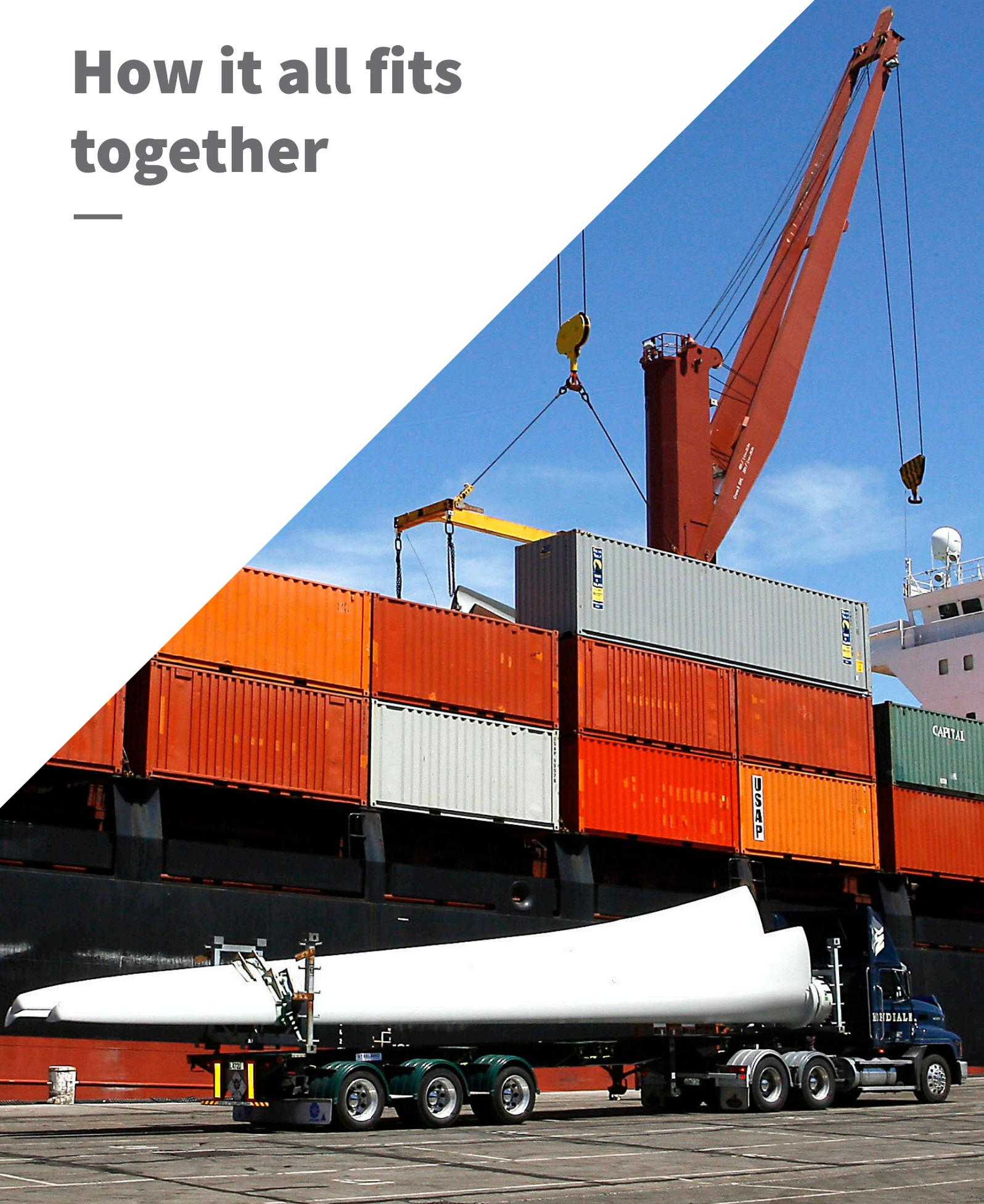
Loading wind turbine blades onto MV American Tern at Lyttelton. Meridian and Antarctica NZ built the three tower wind farm with support and logistics from USAP. Renewable energy now supplements Scott Base and McMurdo Station, cutting fuel consumption by ~463,000 litres and saving 1,242 tonnes of CO<sup>2</sup> annually. Photo: Scott Bennett
